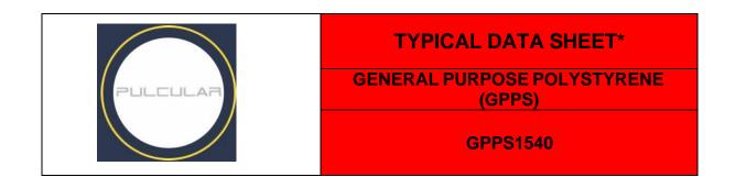
GPPS1540 is easy flowing crystal polystyrene designed for extrusion or injection applications. It improves extruder output and thermoforming cycle time when mixed with a high impact polystyrene such as HIPS7240.It is particularly suitable for glossy-layer co extrusion. This grade has food contact approval.
